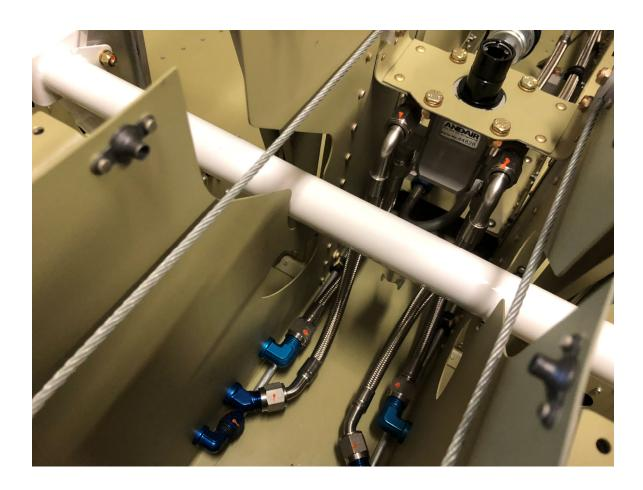
Below is an image of a mounting plate that was fabricated by an RV10 EFII builder utilizing wing root filters. He said it fit well with minimal filing required. This is for reference only...you may need adjustments depending on how you mount it as well as if you are doing SDS Versus EFII
